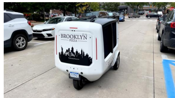
Magna-developed autonomous all-electric last mile delivery robot at work in urban environments in Michigan.
