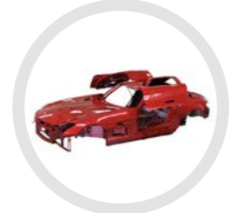
Mercedes-Benz SLS AMG Aluminum body (2009 – 2014)
