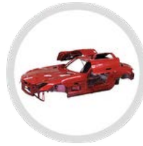
Mercedes-Benz SLS AMG Aluminum body (2009 – 2014)
